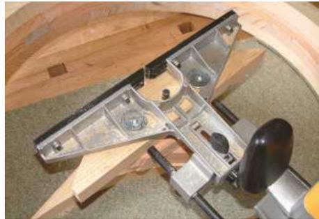
▲ Pic.9 Screw a piece of wood to the router fence and drill an 8mm hole, the trammel centre
